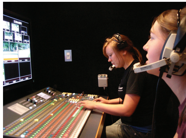
FIGURE 1.8 Production switchers are used to switch between two or more live cameras during a project.
